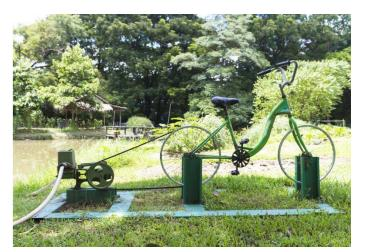
Four AUAS technology students designed a vegetable, fruit and garden waste shredder to feed the first underground worm container in Netherlands. The standard worm hotel has been ineffective due to big temperature fluctuations above ground and the large size of the materials fed to the worms. More students and researchers are involved with other innovations coming out. Let's get universities to support us directly
